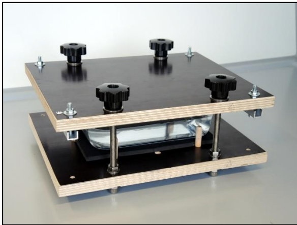
Fig.: After placing the lid on top, the holding fixture is screwed together using the star grip nuts and then turned upside down.
