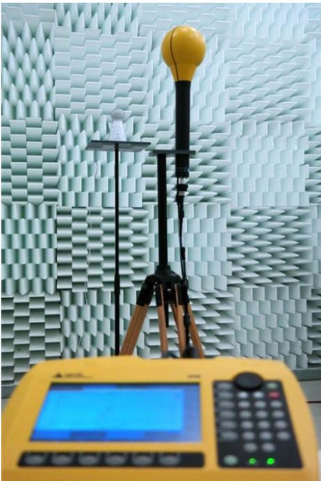
First, the frequency and transmission behaviour in the different operating states (see Paragraph 1.4 Begriffsbestimmungen) of standby mode, standby mode incl. connectivity check and active mode is determined. The operating states are achieved here using suitable settings or applications (e.g. external noise source).
