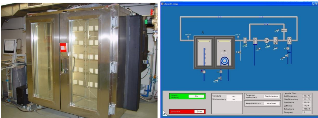
Figure 2: Photograph of the accelerated weathering chamber during operation (left) and a screenshot of the monitoring program (right). (©Fraunhofer IBP)
