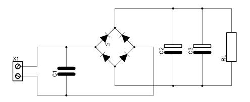
Test setup as test load for measurements 6 to 8
