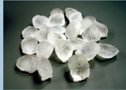
*The material that makes Rhepanol roofing membranes so special: Polyisobutylene (PIB).*
