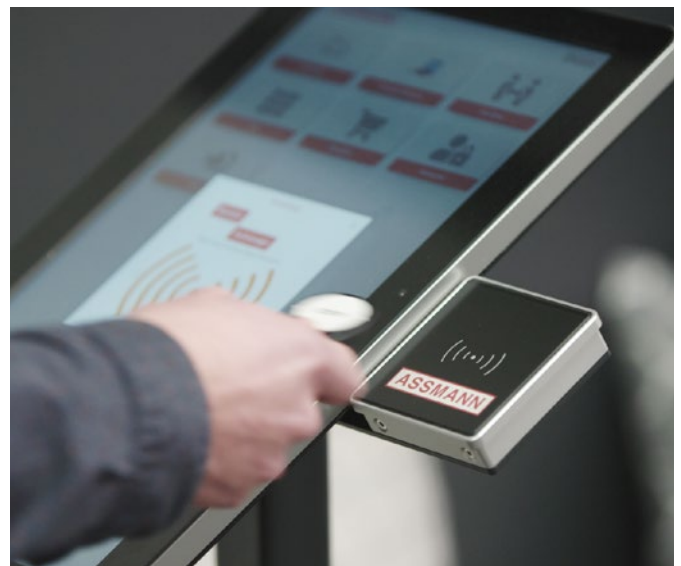
Log-in: RFID chip cards to open the lockers
