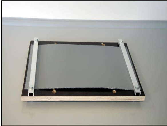
Fig.: The glass bowl is placed onto a soft underlay and held in position by wooden pegs. The roof sheet is fixed to the board using two aluminium rails. This ensures precise positioning of the glass container on the same section of the roof sheet after replacing the water.
