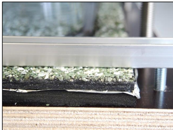
Fig.: For roof sheets with a rough surface, the rough layer of the sheet where the rim of the glass container touches the roof sheet is cut away. A soft aquarium mat is also required underneath the roof sheet for sealing purposes. An intermediate layer of aluminium foil is used to separate the two materials.
