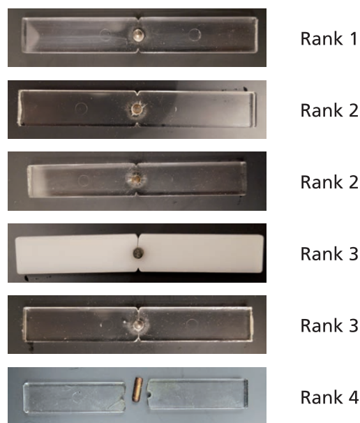
Fig. 3 Assessment of stress cracking corrosion for selected types of plastics.
